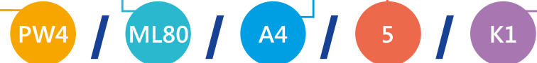
Piston manifold 4-ways "pulse free", liquid diam gauges. 80, for R410a/R32, connections 5/16"SAE, class 1
